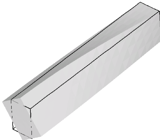
Figure 10: First torsion mode
